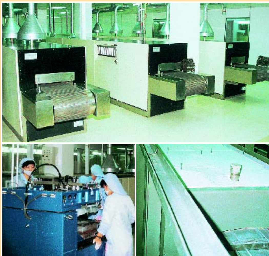
Fig. 34. FIBROTHAL modules used in a conveyor belt furnace
