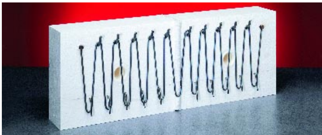
Fig. 5. ROB with free-radiating heating elements for a maximum element temperature of 1300°C, mainly for wall and floor heating
